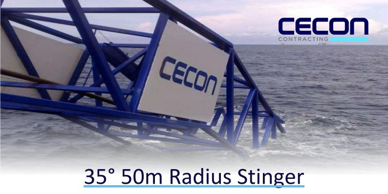
Cecon Contracting's smaller modular stinger provides pipe support from the deck to the natural caternary during lay. Designed for rigid pipe up to 6" (water depth and wall thickness dependent) in S lay configuration, this modular stinger is easily mounted on board a vessel, and pivots out of the water during transit. Pairs well with Cecon Contracting's 36t tensioner.
